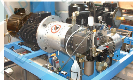
Maintenance-free sealing of proportioning pumps for polyol and isocyanate in high-pressure reaction moulding machines
